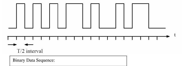
b. Now assume that the waveform represents differential Manchester coding, and find the two possible bit streams.
